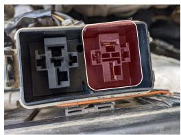
Remove relay, add relay bypass
